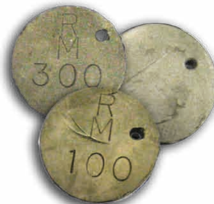
Swollen rubber elastomeric coupons tested in a Methyl Pyrrolidone solvent (photo courtesy of Eastman Chemical Company)
